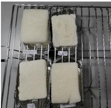
Figure 2. 4. Schematic representation of special setup used to thaw food simulants
